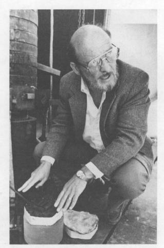
PAUL COOPER (DMTS, 9333) explains the half-scale test apparatus used for impact-ignition experiments. Small black cylinders near his left hand are propellant pellets, which are arranged on a large plastic cylinder that simulates the mechanical properties of more layers of pellets.
